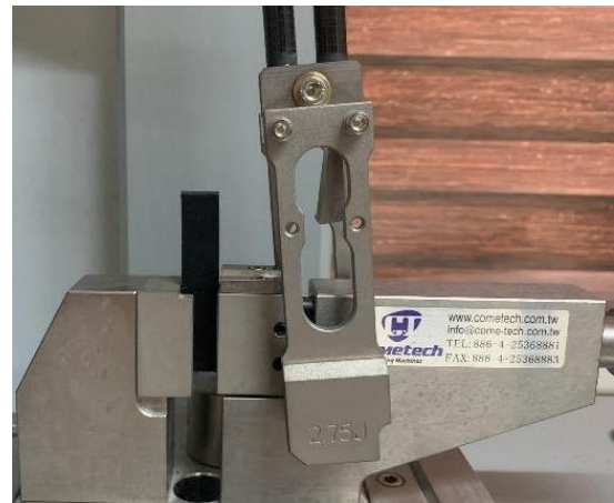
Figure 6. Actual Impact Test Set-up
