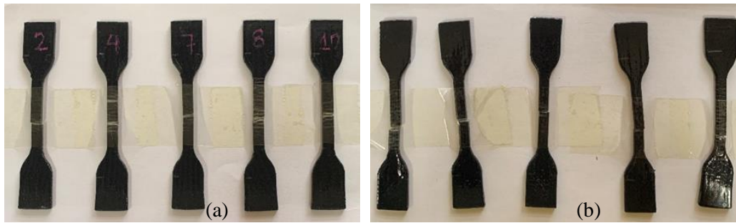
Figure 10. (a) Unpolished and (b) Polished Type IV Tensile Specimen
