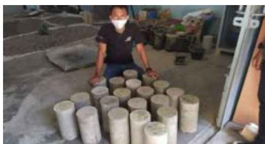
Figure 5. Cylinder samples of concrete.
