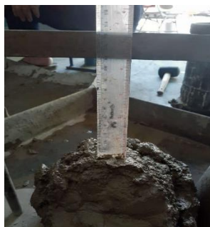
Figure 4. Slump test process to concrete
