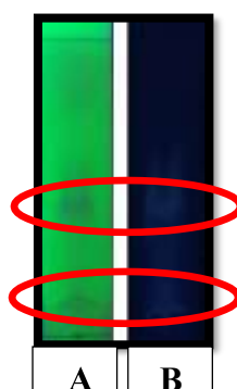
Figure 2. KLT profile of ethyl acetate extract of Bajakah Buton (Kakatola) root. A) under UV light 254 nm; B) under UV light 365 nm
